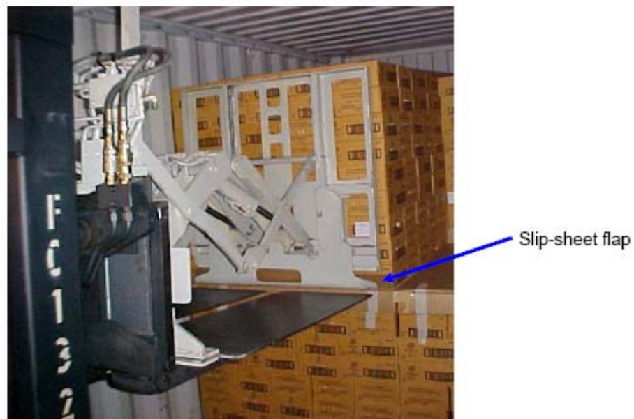
Figure 14. The photo above shows a forklift with a slip sheet attachment preparing to pull a Ti-Hi onto its tines.
