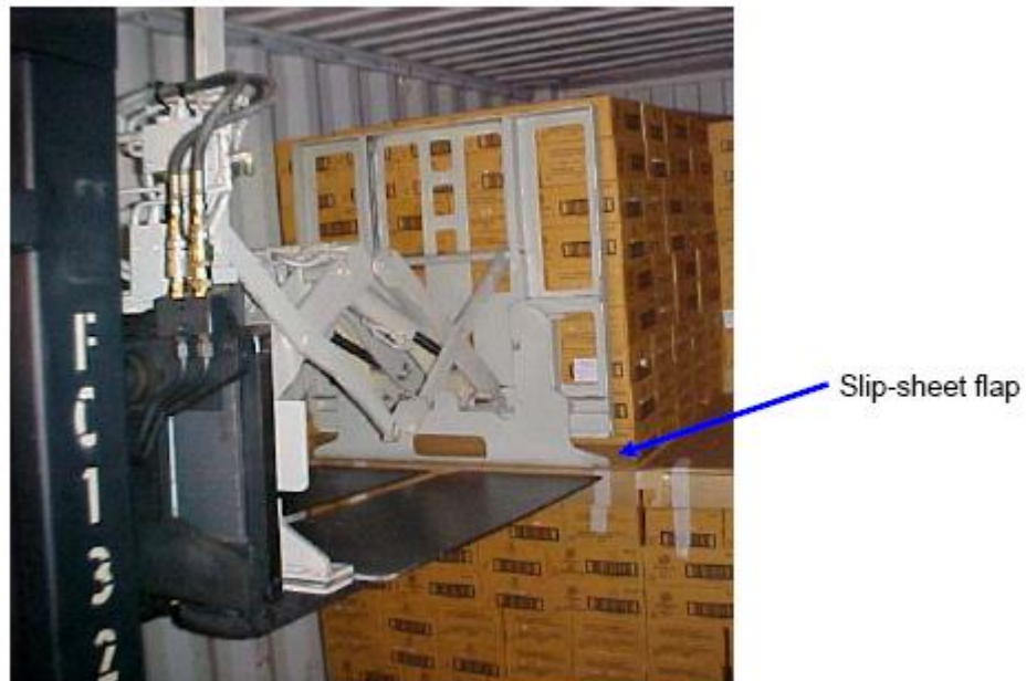
Figure 15. The photo above shows a forklift with a slip sheet attachment preparing to pull a Ti-Hi onto its tines.
