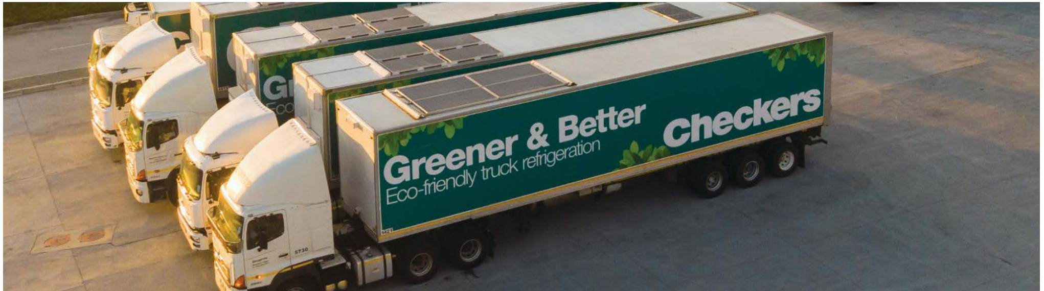
The solar panels on the roofs of these trucks keep their contents cool and reduce GHG emissions.
